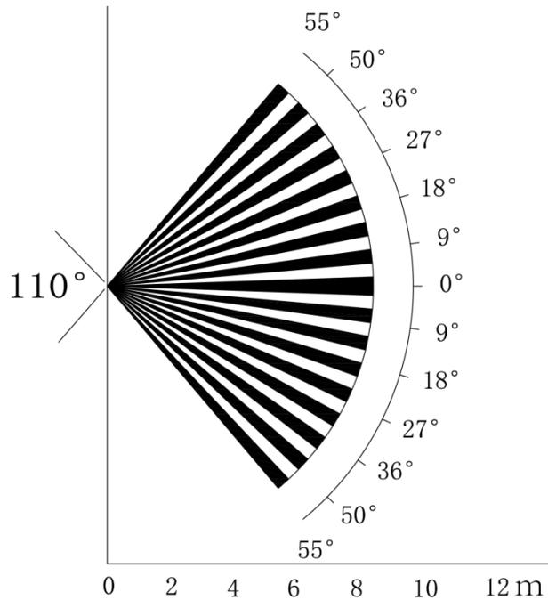
For model A and B, the vertical detection distance of the sensor is 2 m–10 m. For model C, the distance is 1 m–12 m. See Figure 3-2.
